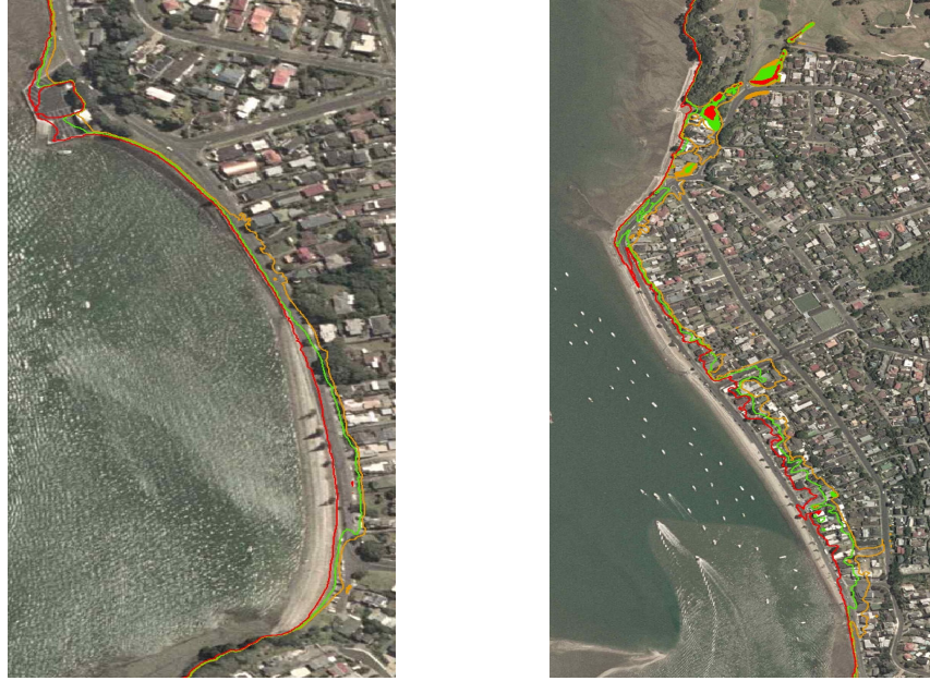
Figure 8: 1% AEP storm-tide contours for the present day (red), 2050's (green) and 2080's (orange) for the Bucklands Beach (southern part (left) and northern part (right)).
